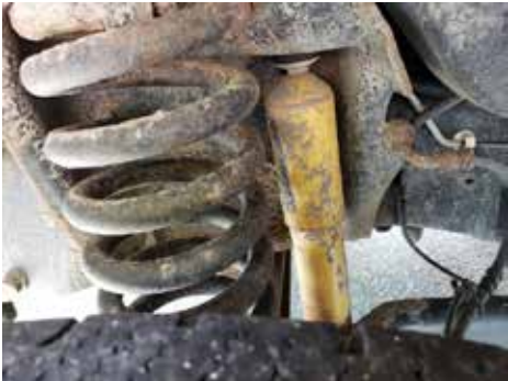
SCS: Undercarriage corrosion
