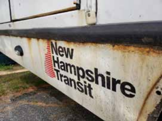
SCS: Corrosion on lower panel/wheel well
