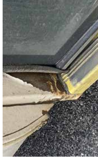
VNA@HCS: Corrosion affecting passenger door
