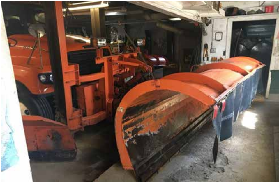
View of the front of truck with plow equipment mounted and parked in shed. Minimal clearances and uneven surfaces throughout the building make it difficult to navigate and increase risk of accidents and injuries.
